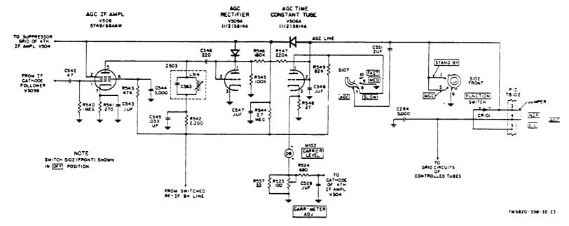
The AGC's of many R-390A's, including mine, have been modified using the so-called Cornelius AGC mod which was described in HSN 1 and 10. The mod consists of removing R545, replacing R546 by a 1N34A, 1N60, 1N270, 1N914, or 1N4158 diode with cathode connected to pin 1 of V509A, and replacing of R547 by a 10K ohm half watt resistor. The mod increases the AGC line voltage, which reduces the signal level at the diode detector V506B and, consequently, improves SSB reception quality.
